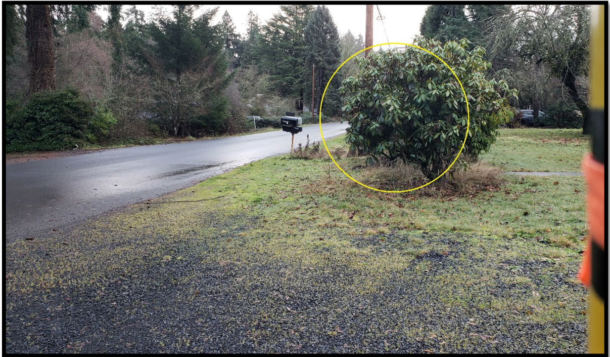
Figure 2: Sight Distance to East of Access Driveway: On-site Bush to be Removed
